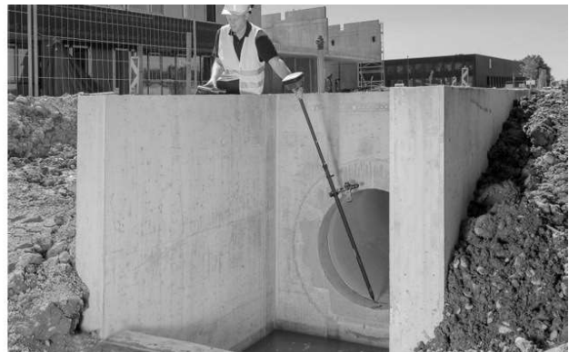
Figure 3 - Using the Leica GS18 T to measure building corners and obstructed points that were previously not measurable in conventional RTK surveying with a vertical pole.
