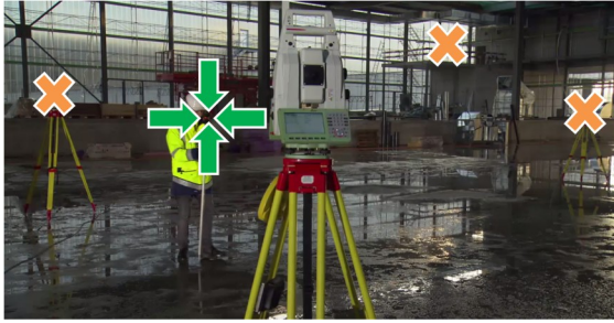
Figure 16 - Using the PowerSearch filter to eliminate non-relevant targets.
